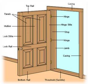
**Outside Hinges:** Doors with hinges on the outside will give a burglar easy access to your home. The burglar only has to remove the hinge pins and lift the door from the frame. This can be corrected in three ways:
